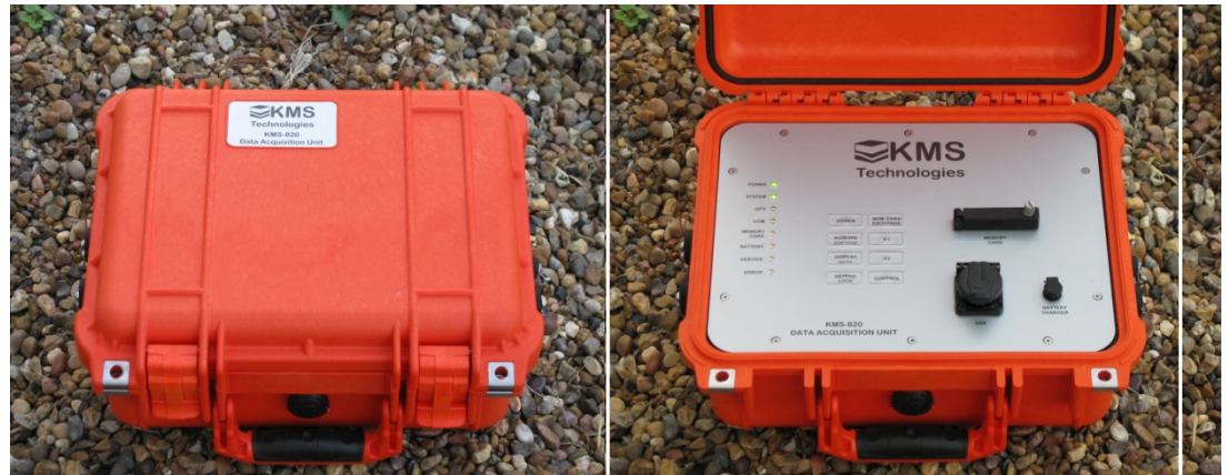
KMS-820 data acquisition unit.
